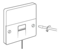
5. Carefully unscrew the 2 small screws and the bottom half of the faceplate should slide out. On the right-hand side is a test socket. This connects you directly to the telephone line and bypasses any extension wiring you may have.
